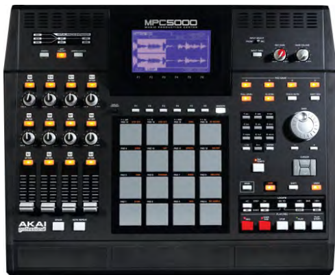
Figure 5. Akai MPC 500 with “Chop Shop” waveform slicing activated. Regions of the waveform seen in the display can be played back directly from the grey pads in the middle of the device [9].
