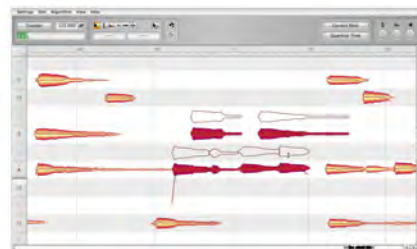
Figure 3. A waveform that has been split into its tonal components and mapped to a piano roll representation in Melodyne DNA [10].
